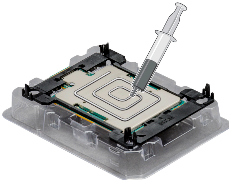
Figure 34. Applying thermal grease on top of the processor
