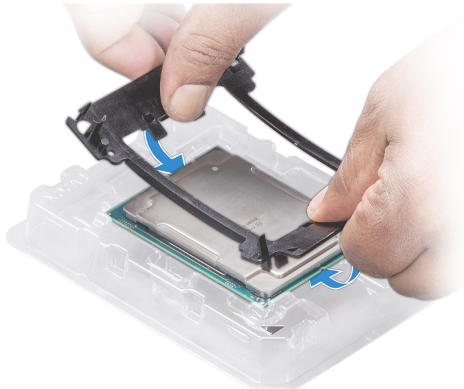
Figure 40. Installing the processor bracket
