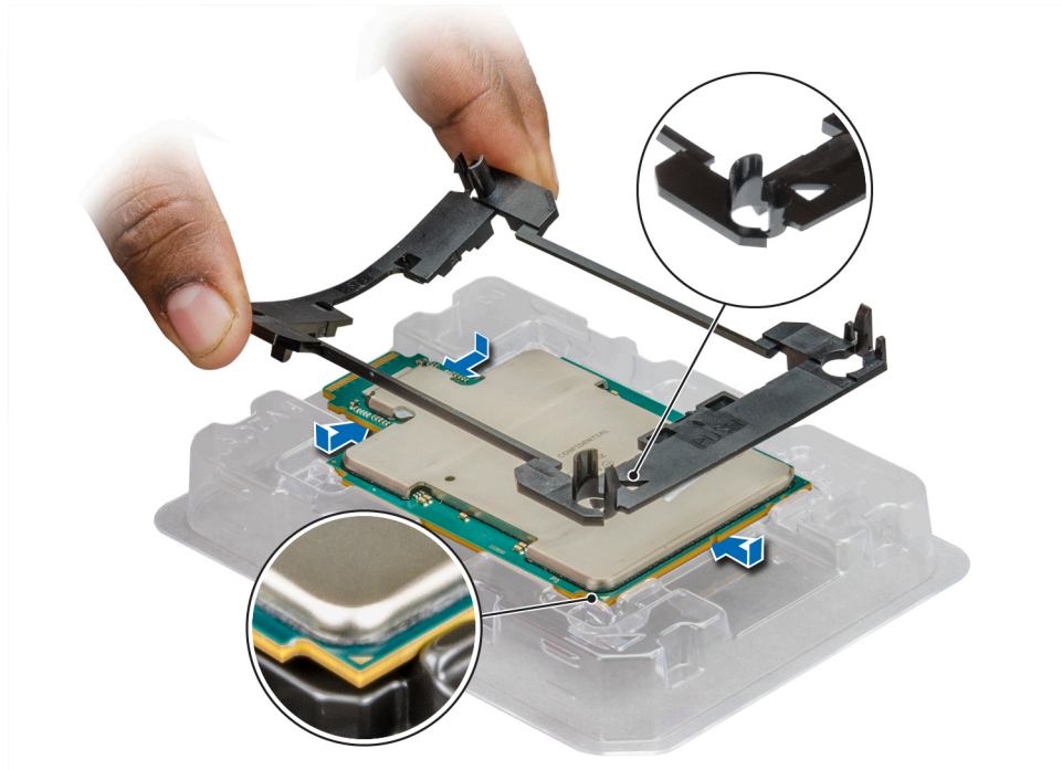
Figure 33. Installing the processor bracket
