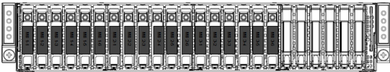
Figure 10. 2.5-inch drives (24) with three C6520 sleds
