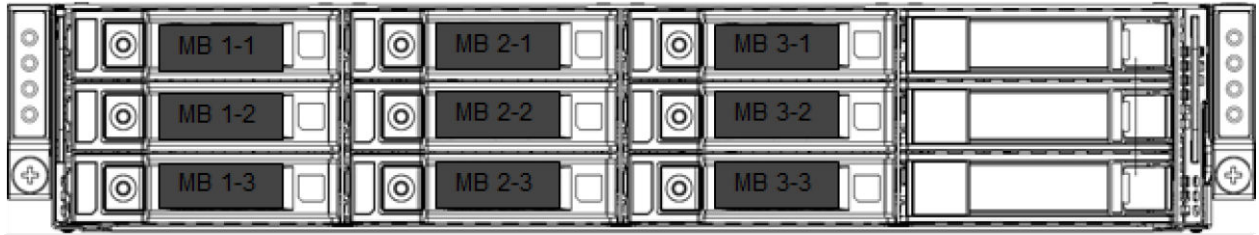
Figure 20. 3.5-inch drives (12) with three 1U sleds
