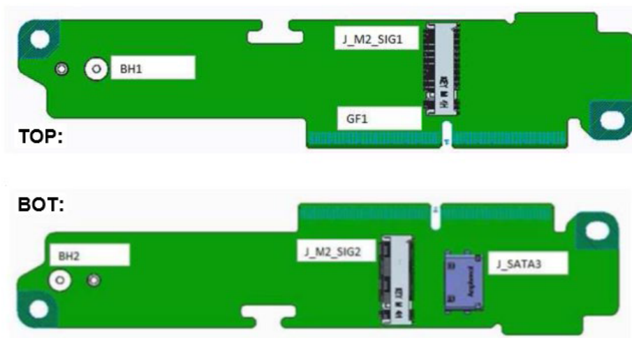
Figure 8. M.2 X 16 SATA Riser PCB Dimension
