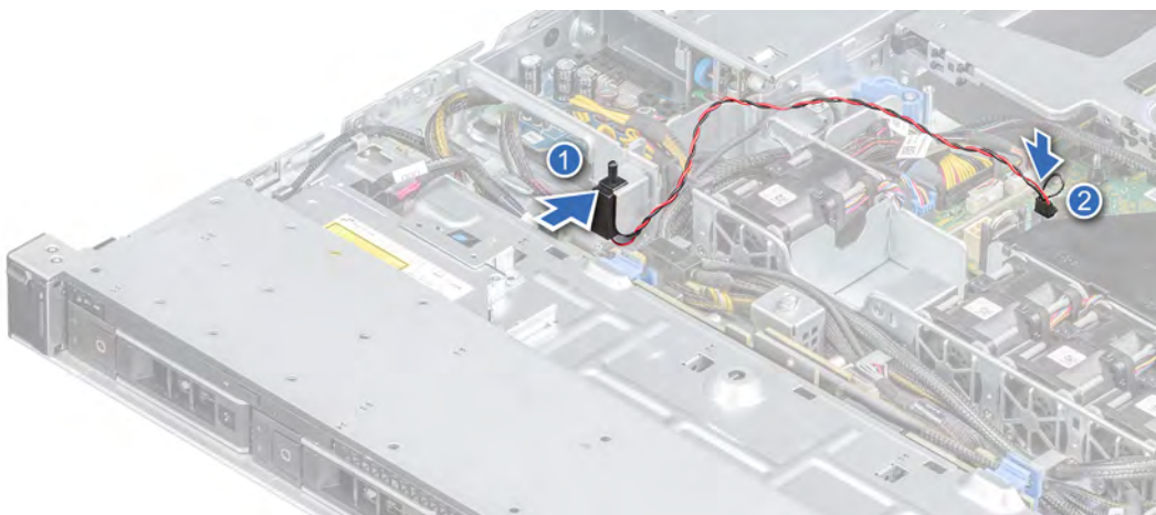
Figure 32. Installing the intrusion switch
