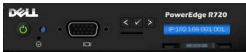
Figure 9. R720 LCD control panel
