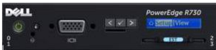
Figure 9. R730 LCD control panel
