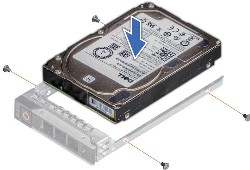
Figure 54. Installing a drive into the drive carrier
