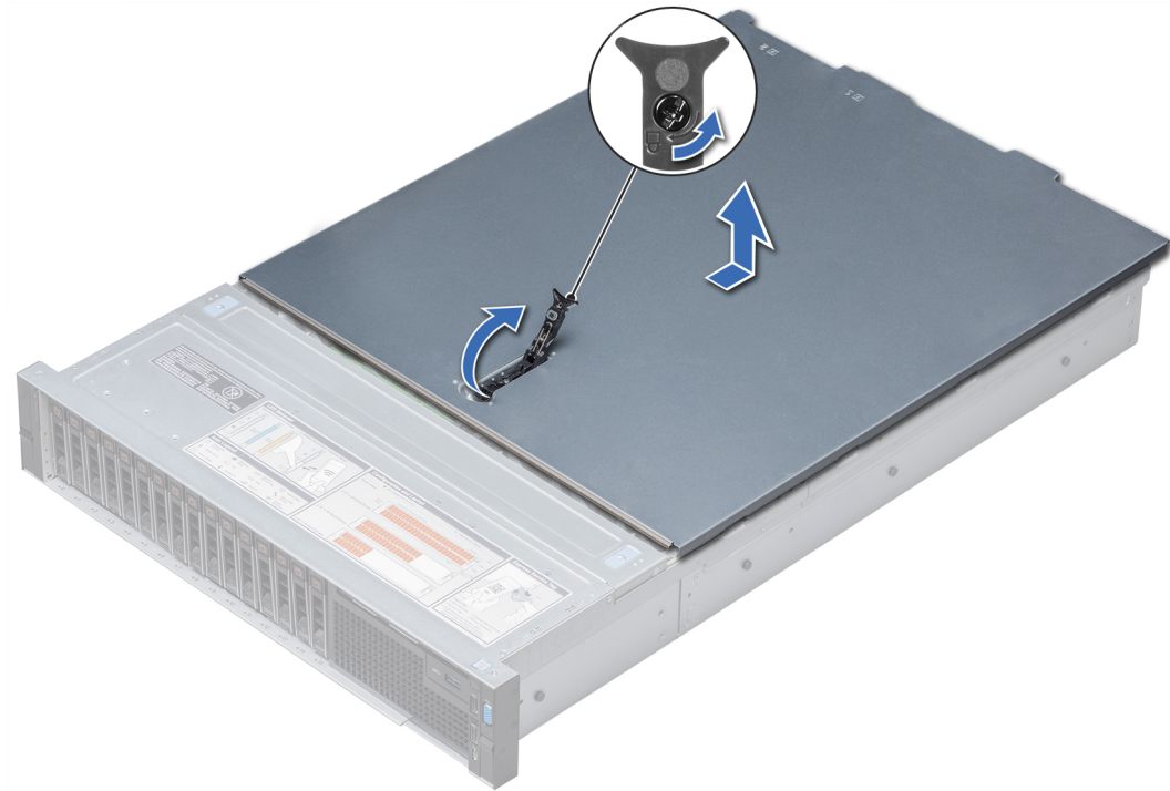
Figure 25. Removing the system cover
