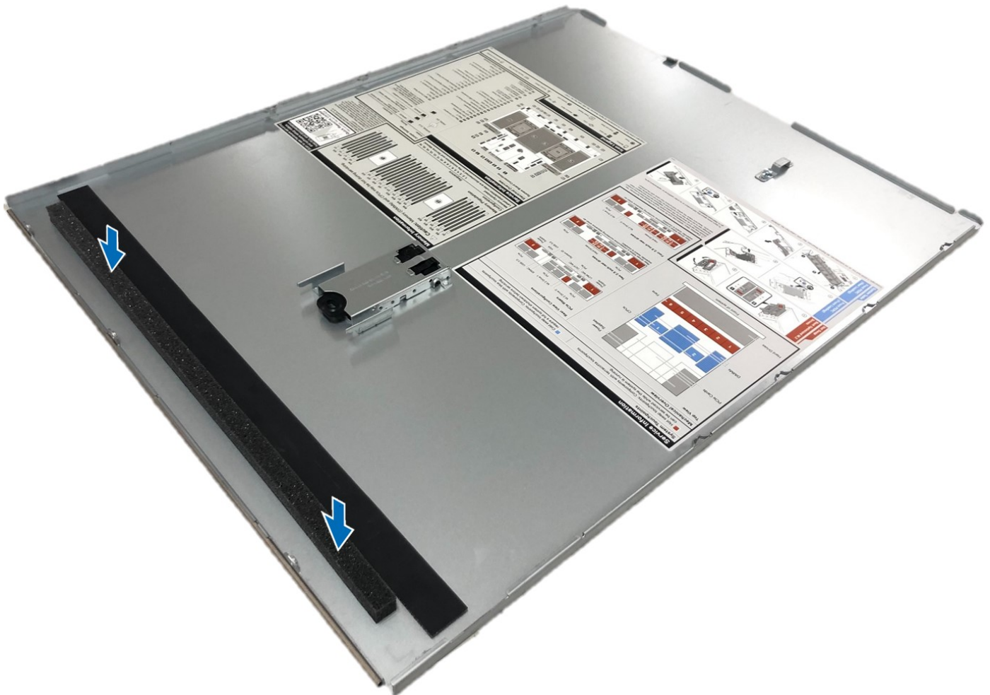
Figure 232. Installing Mylar foam on the system cover
