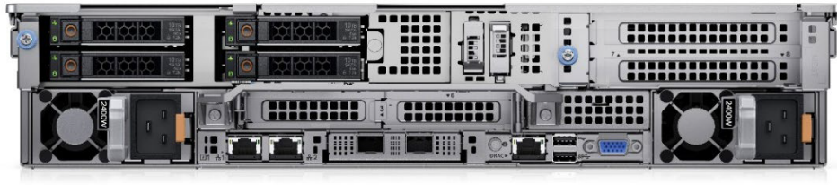
Figure 12. Rear view of the R750 with 4x 2.5 inches storage drives, 4x PCIe Gen4 slot and Hot-plug BOSS
