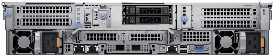
Figure 10. Rear view of the R750 with 2x 2.5 inches storage drives, 6x PCIe Gen4 slots and Hot-plug BOSS
