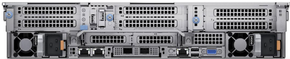
Figure 11. Rear view of the R750 with 8x PCIe Gen4 slots and Hot-plug BOSS
