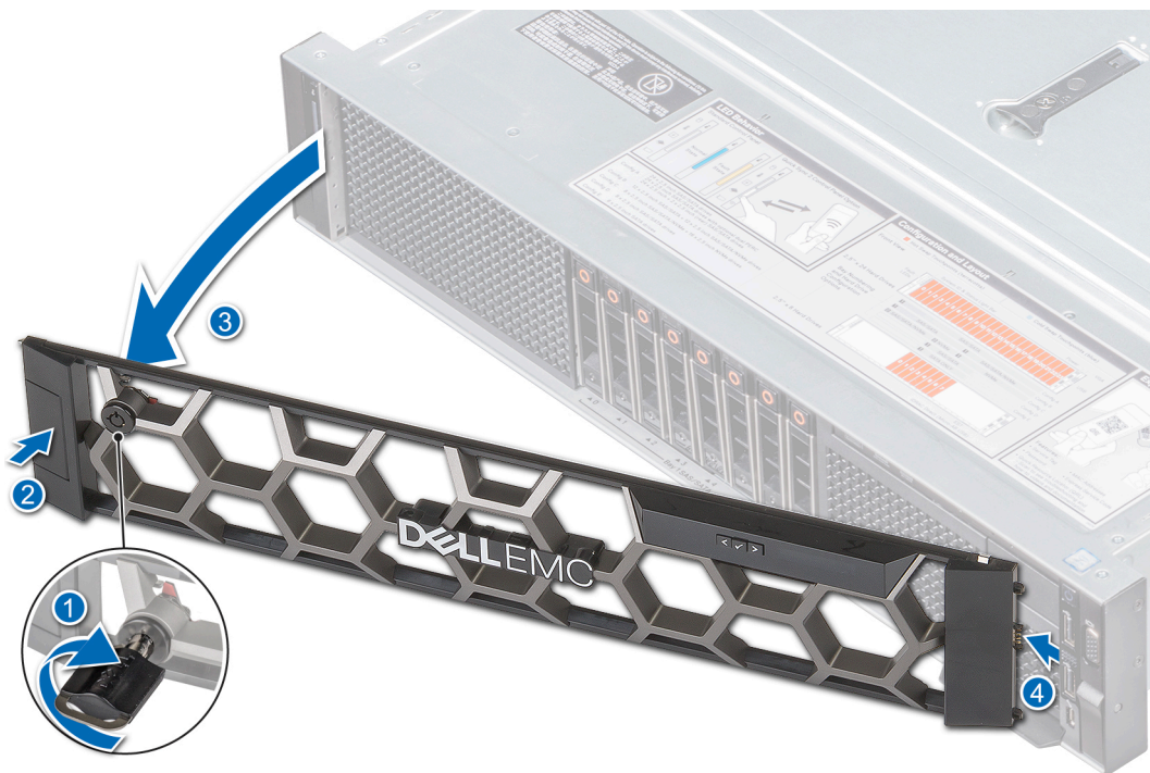
Figure 17. Removing optional front bezel
