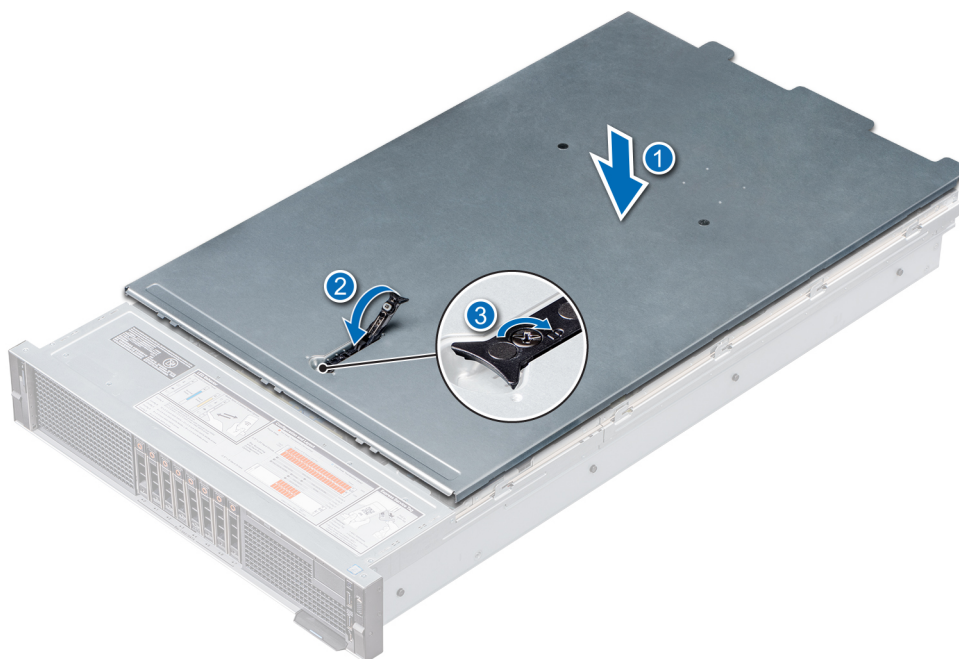
Figure 20. Installing system cover
