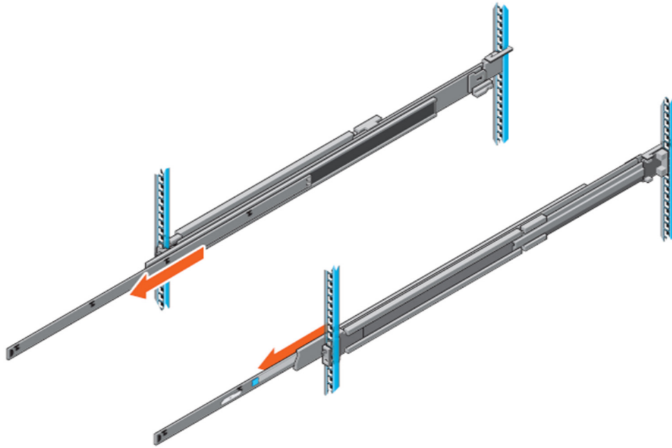
Figure 28. Pull out inner rail
