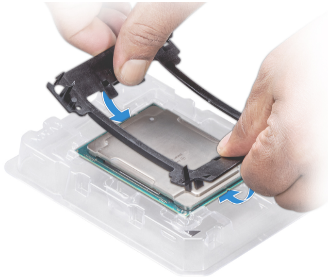
Figure 17. Installing the processor bracket
