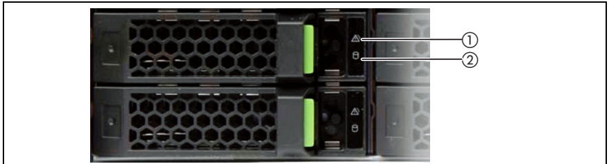
Figure 16: Indicators on the 3.5 inch HDD modules
