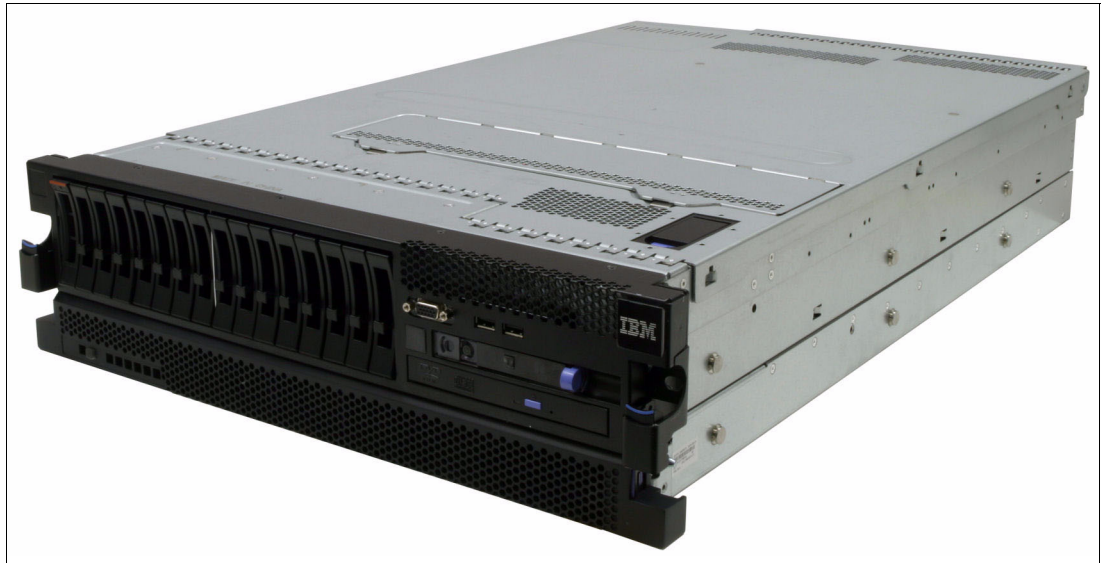
Figure 4-5 x3690 X5 with the attached MAX5 memory expansion unit
