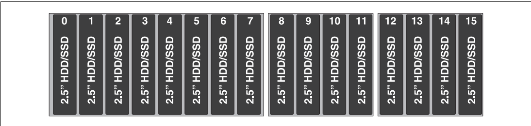
Figure 4-36 x3690 with one 8x 2.5-inch backplane and two 4x 2.5-inch backplanes
