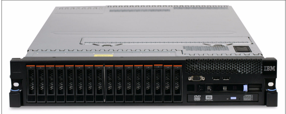
Figure 4-19 Front of the x3690 X5 with sixteen 2.5-inch drive bays
