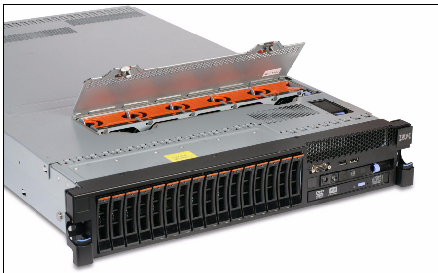
Figure 4-48 Hot-swap fan access panel
