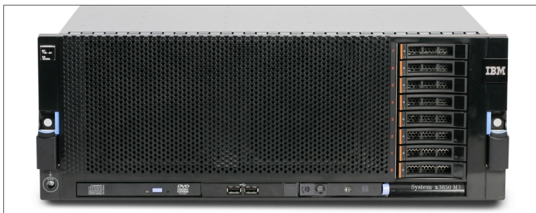
Figure 3-24 Front view of the x3850 X5 showing eight 2.5-inch SAS drives
