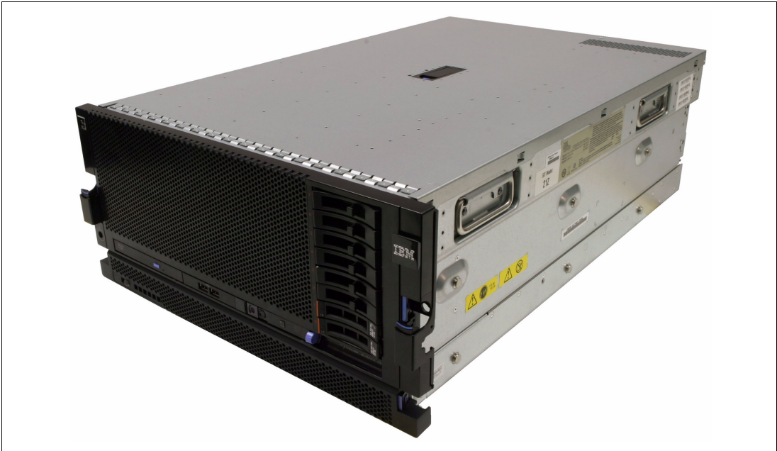
Figure 3-4 x3850 X5 with the attached MAX5 memory expansion unit
